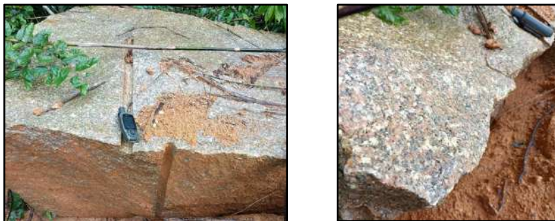
Figure 4: Semi-drill holes in RT from granite block cutting
